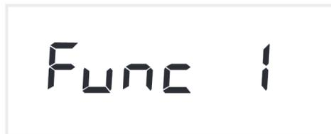
The display will show **„Func“** (function). In this menu the function of the relay is set in connection with the delay function. The value can be changed by using the **„▲▼“** buttons.
