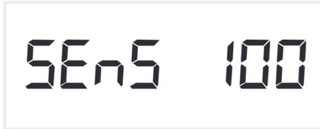
The display will show **"SEnS"** (sensitivity). In this menu the sensitivity of the sensor can be adjusted. Default value is 100 kOhm. The value can be changed by using the „▲▼“ buttons.
