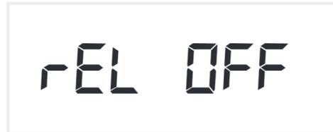
The display will show **"rEL"** (relay). In this menu the starting position (sensor is not activated) of the relay is defined as "ON" or "OFF". Default value is "OFF". The value can be changed by using the „▲▼“ buttons.
